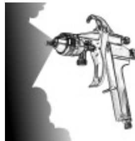
Conventional High Pressure Spray Gun Overspray
